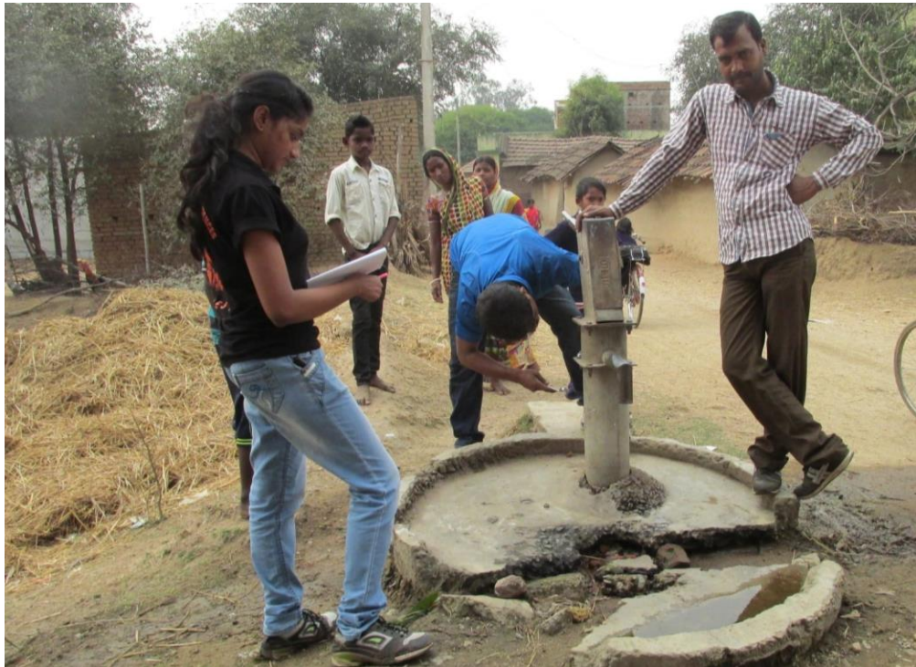
Taking measurement of ground water level from tube well from Barabazar Block, Purulia. Picture Courtesy: Puja Chaudhury
